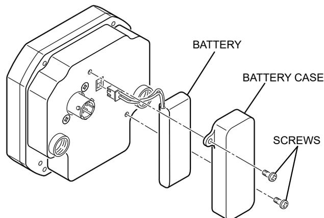
Figure 4.7, Battery Replacement
